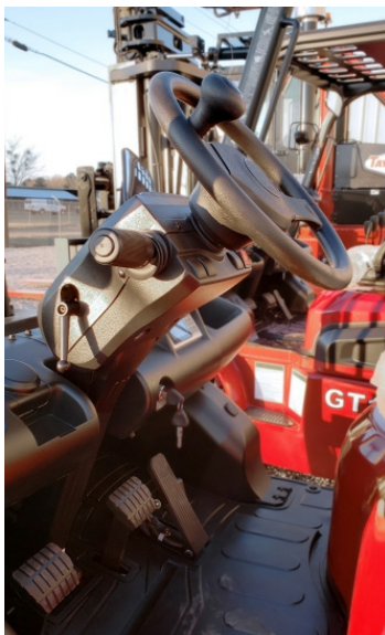
Adjustable Steering Column Pivots 30 Degrees
