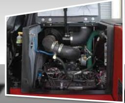
Large, hinged doors provide easy access to engine and transmission daily service points.
