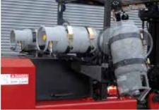
Dual, heavy-duty, swing-out / flip-down mounts for easy removal of LP gas tanks.
