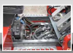
Simple, removable floor plate further adds to the access of the drivetrain.
