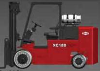
XC-180S & 180SL (SL r (a) 24-in. (6 Rated Capacity 18.000-lbs. (8. n) Load Center Alt. Capacity 16,000-lbs. (7 ) 30-in. (7 1) Load Center Alt. Capacity 14,000-lbs. (6 3) 36-in. (9 n) Load Center m) Wheelbase
