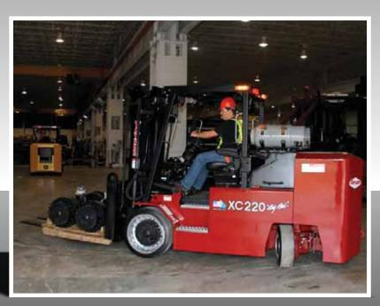
The chassis is 56.5" wide and has a turn radius as tight as 121"...without sacrificing power, operator comfort or stability.
