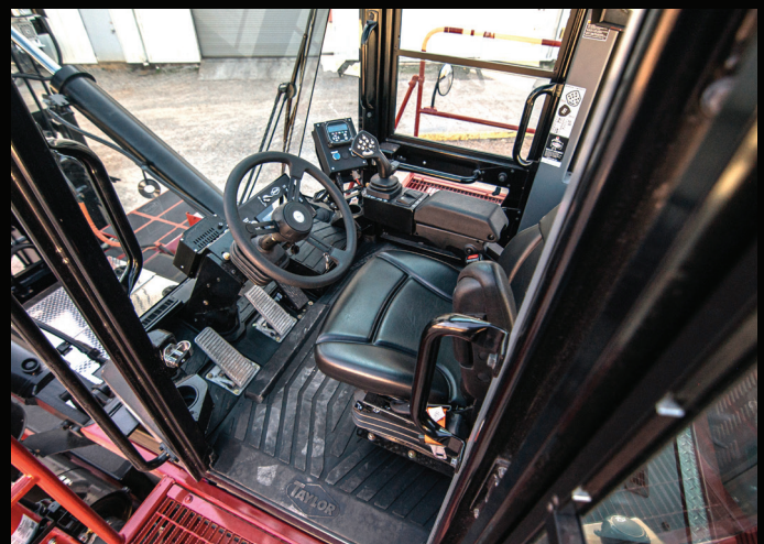
FULLY ENCLOSED 2-DOOR CAB - ALL STEEL - 32,000 BTU HEATER (STANDARD)
